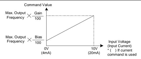
Figure 12 Analog Input Gain and Bias
