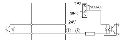
• PNP Sensor (Source) used for operation signal.
