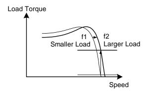
Figure 19 Output Frequency with Slip Compensation.
