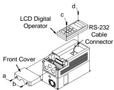
Attach the digital operator and tighten the screws in the place c and d. Insert the tabs on the upper part of front cover into the groove of the inverter and tighten the screws in the place a and b.
