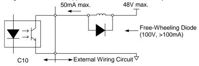
Figure 4 The Optical-Couplers Connect to an External Inductive Load
