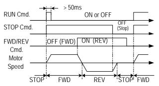
Figure 39 Operation Sequence in 3-wire Mode
