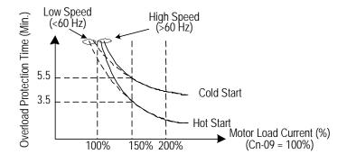
Figure 37 Motor Overload Protection Curve (Cn-09 Setting = 100%)
