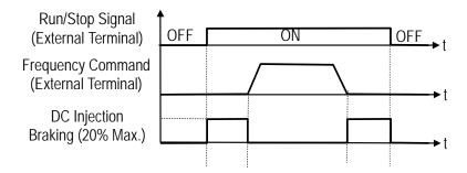
Figure 36 Zero Speed Braking Operation Selection
