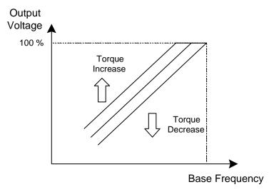
Figure 13 Adjust the Auto Torque Boost Gain Bn-11 to increase the output torque.
