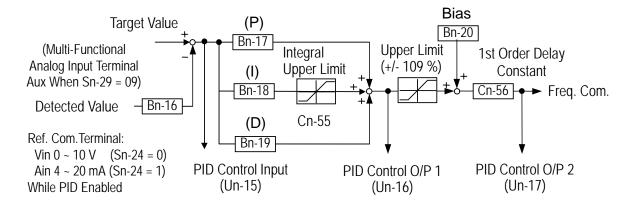
Figure 14 Block Diagram for PID Control in C10
