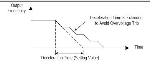
Figure 35 Stall Prevention Function During Deceleration (Sn-15= 1)
