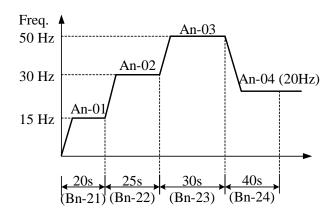
• Sn-44 = 1~3: If the inverter stops and restarts again, it will continue running from the unfinished step, according to the setting of Sn-44.
