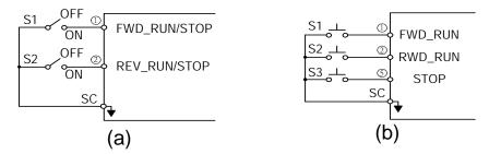
Figure 402-wire Mode Connection Diagram
