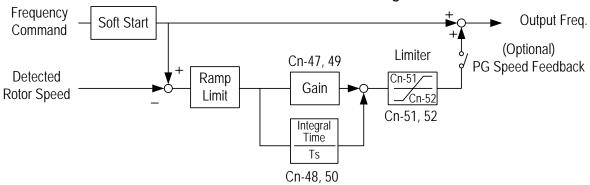
Figure 44 PG Speed Control Block Diagram
