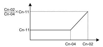
Figure 20 Slip Compensation Limit
