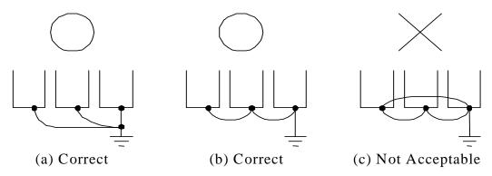
Figure 5 Grounding of C10 Inverters.
