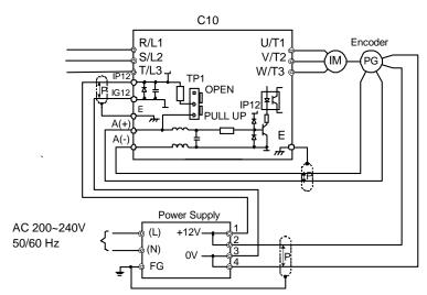
Figure 50 Wiring of PG feedback
