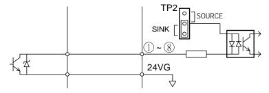
NPN Sensor (Sink) used for operation signal.
