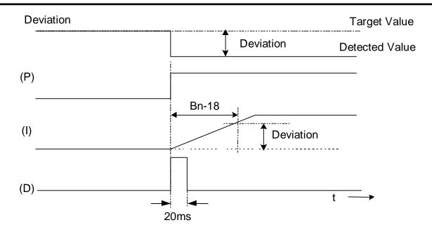
Figure 15 Response of PID Control for STEP-Shape (Deviation) Input
