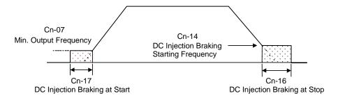
Figure 21 DC Injection Braking Time Chart
