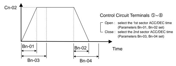
Figure 11 Acceleration and Deceleration Time
