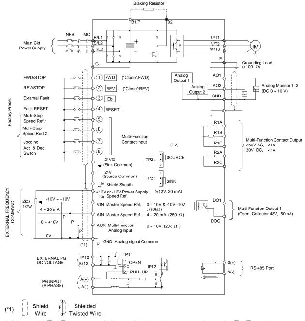
(\*2) The terminal (1) ~ (8) can be set as SINK or SOURCE type input interface, when setting (1) ~ (8) as sink type input, the short jumper of TP2 must be set to SINK position, and set to SOURCE position for source type input.
