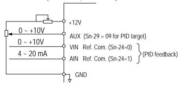
Figure 49 PID Wiring Diagram
