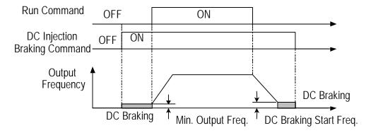
Figure 43 Time Chart for DC Injection Braking Command
