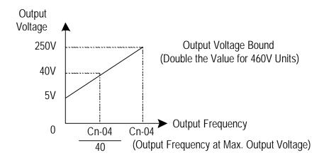
Figure 34 Output Voltage Limit
