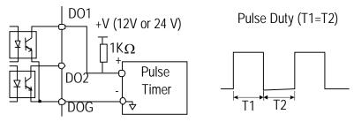
Figure 46 Pulse Signal Output
