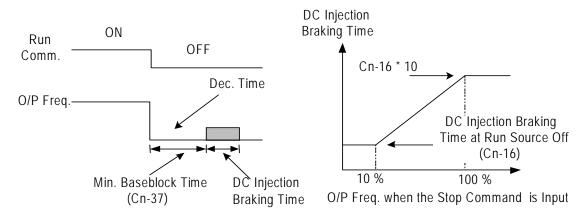
Figure 32 Whole Range DC Injection Braking Stop
