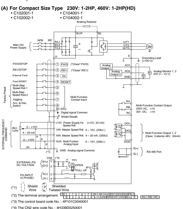
Figure 2-a Standard Connection Diagram
