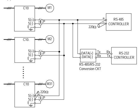
Figure 51 Wiring for MODBUS Protocol Communication
