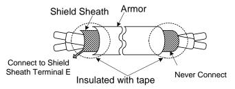
Figure 3 Shielded Wire Termination
