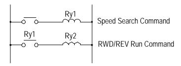
3. When the Speed Search and DC Injection Braking are set, set the Min. Baseblock Time (Cn-37). For the Min. Baseblock Time, set the time long enough to allow the motor's residual voltage to dissipate. If an overcurrent is detected when starting a Speed Search or DC Injection Braking, raise the setting Cn-37 to prevent a fault from occurring. The Cn-37 setting cannot be set too small.
