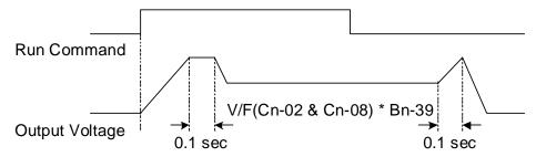
Figure 17 Time Chart for Energy Saving Operation
