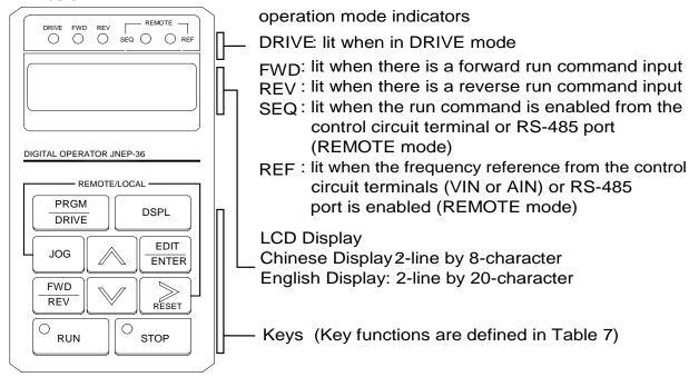
Figure 10 LCD Digital Operator
