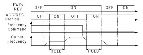
Figure 42 Acceleration and Deceleration Ramp Hold
