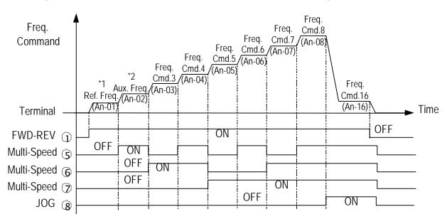
• Figure 41 shows the operation sequence of a multi-step speed and jog command.
