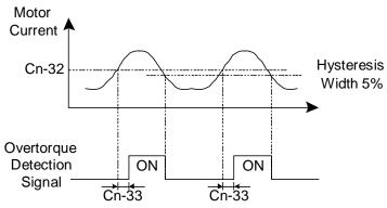
Figure 26 Overtorque Detection Time Chart
